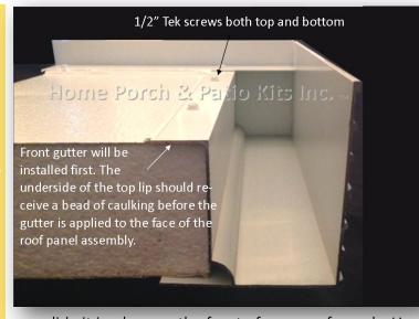
With all your roof panels in place and secured properly, measure the exact length of front gutter assembly you will need. This is the outside edge to outside edge measurement of your panel assembly. If you have more than 24' you will choose a place along the width that will have a butt-splice of the two pieces coming together. This seam will need to be caulked.
