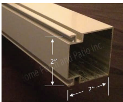
H122 - 2" x 2" Mainframe .048" wall thickness (H120 corners = .062" wall thickness)
